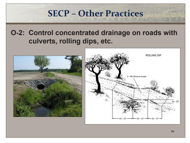
O-2: Control concentrated drainage on roads with culverts, rolling dips, etc.
