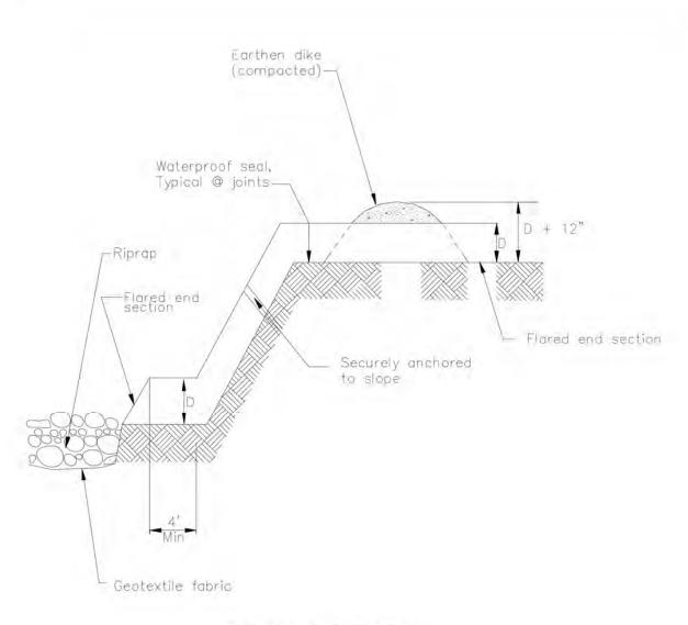
TYPICAL SLOPE DRAIN NOT TO SCALE
