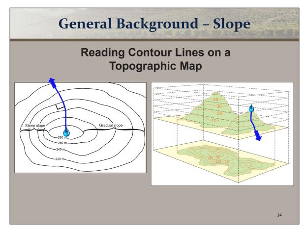
Contour lines describe the elevation of a site on a topographic map. The intervals between the contours can vary. In the image on the left, the interval is 20 meters. In the image on the right, the interval is 10 unknown units. Although the units are unknown, the trend is still increasing as the circles reach inward to develop the peak.
