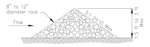
TYPICAL ROCK CHECK DAM SECTION
