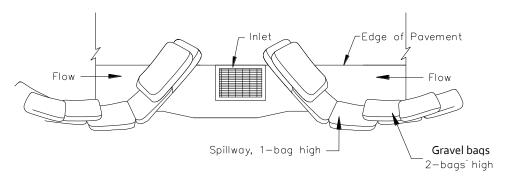
TYPICAL PROTECTION FOR INLET ON SUMP
